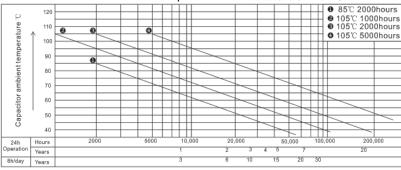
Example: When a 2000 hours/105℃ guaranteed products is used continuously at 60℃, it can be expected to have a life of 5 years. 示例:对于 105 2000 小时的产品,如果在 60 环境中连续使用,它的估算寿命约为 5 年。
